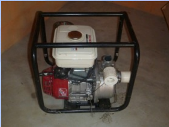
Water pump – 4 horsepower motor
